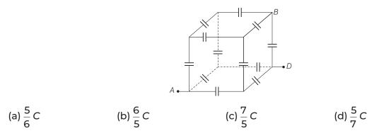
**11.** Find the equivalent capacitance between A and B. A = area of each plate, d = separation between plates
