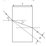
The emergent ray is parallel to the incident ray but displaced sideways by a distance d. If the angles are small, then d is
