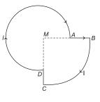
MA = R and MB = 2R, with  $\angle DMA = 90^{\circ}$ . The magnetic field at the centre of the loop is  $\frac{\mu_0 I}{2}$
